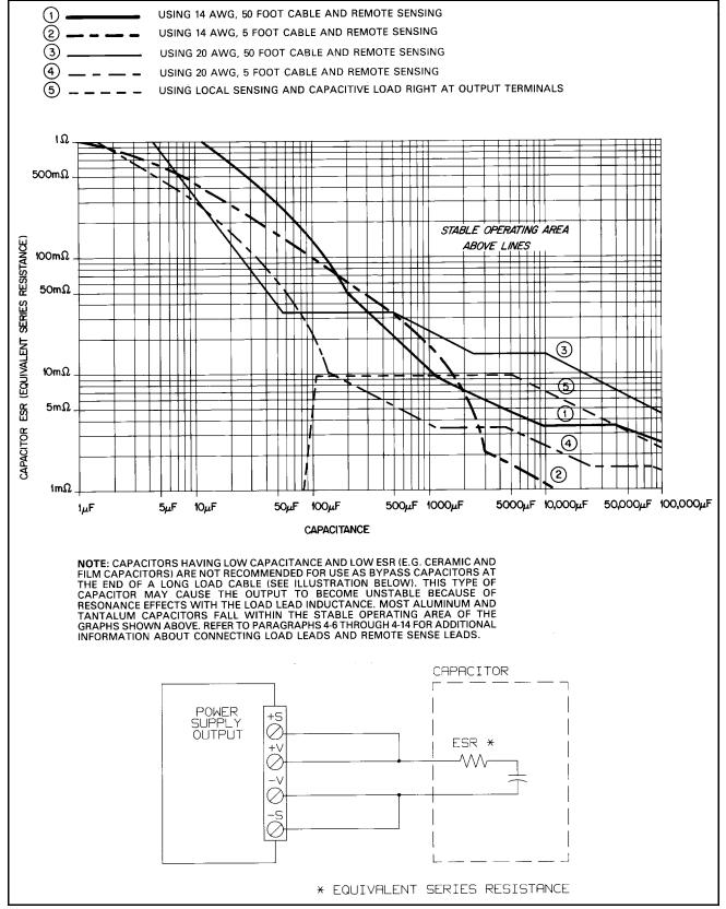
Figure 1-4. CV Operation with Capacitive Load, Stability Graph for all Outputs
